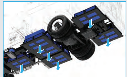
TWO TO SIX TIMES MORE BATTERY POWER—316 KWH TOTAL CAPACITY WITH UNDERSIDE REMOVAL ACCESS
